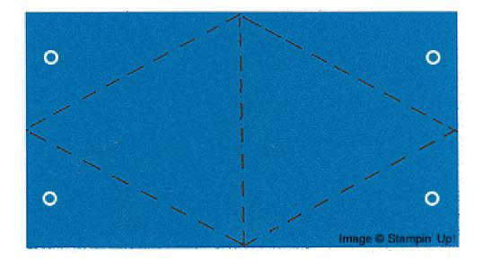
To create a larger triangle box, simply start with a larger rectangle. Divide the length in half, and the height in half, to find the scoring points.
